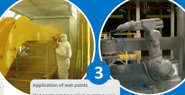
Wet paints can be applied in various ways. They are appropriate for dipping method, robot application, as well as for manual application with a spraying gung, which is the most frequently used method. In cases with bigger work pieces which are difficult to reach, we also manufacture and install lifts, developed by our experts.
