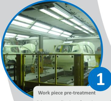
Prior to application of coatings, work piece surfaces have to undergo a pre-treatment process, which enables a qualitative surface protection. The pre-treatment process depends on individual customer's desires. Our lines incorporate systems for chemical pre-treatment on the basis of spraying or dipping, mastic application chamber, grinding and polishing chambers etc.
